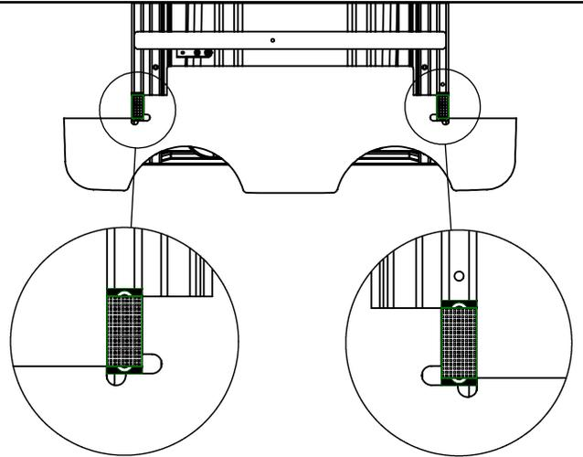
**Place the glass top on the frame using the alignment templates as a reference.**
