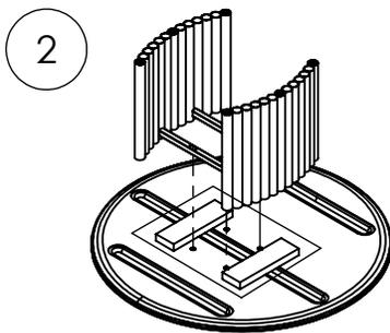
**Place the base on the top and align the holes.**
