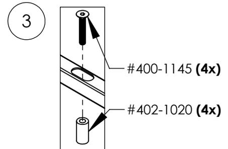
**Insert the screws through the tubes, then put on the spacers.**
